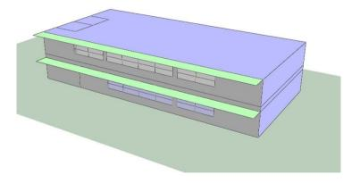
Figure 2: Modified geometry of natural ventilation solution incorporating 2m deep shading on southern windows.
