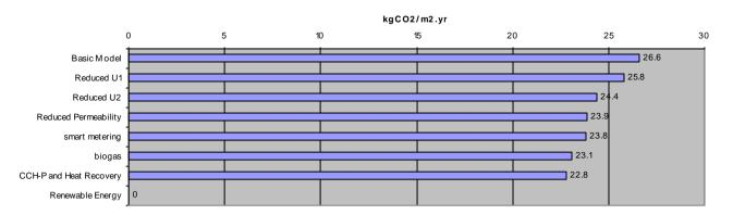
Figure 5: Building Emissions Rates of design stages of the Mechanical Ventilation design strategy
