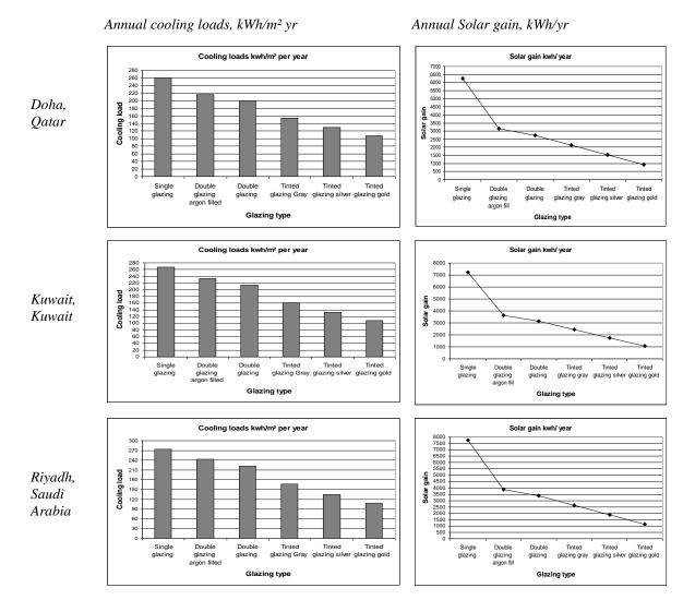
Fig. 3: the effects of changing glazing types on the cooling loads and solar gain in hot climates
