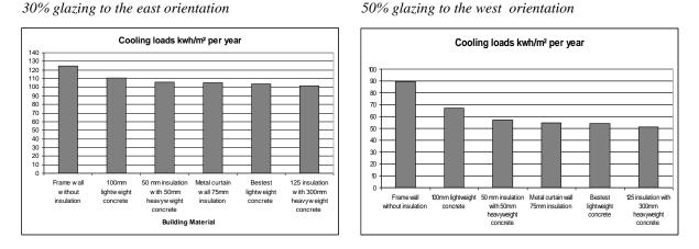
Fig. 5: effects of changing U-value and building materials on the cooling loads
