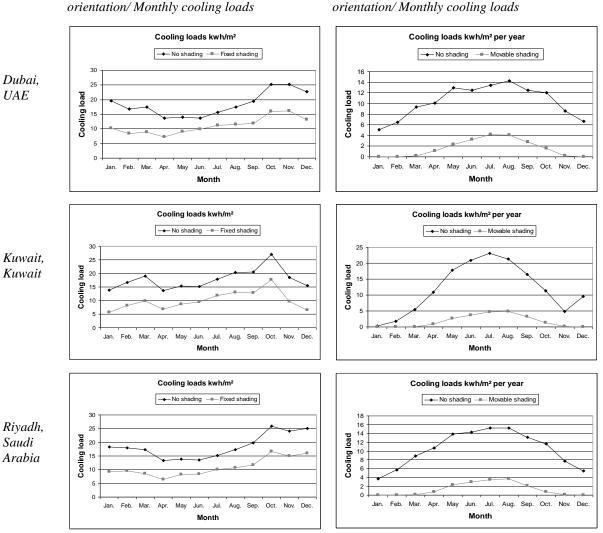
Movable shading, 30% glazing and west orientation/ Monthly cooling loads
